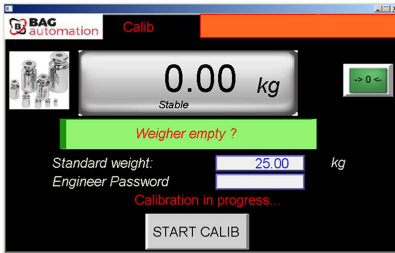
Figure 36 - Calibration: Empty Weigher Acknowledge
